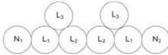
Figure H.52.3 – Special configuration for 6 parallel single-core cables in trefoil (see 523.7)
